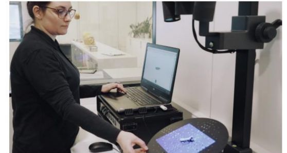
Fig. 4: Quality control with ATOS Q
